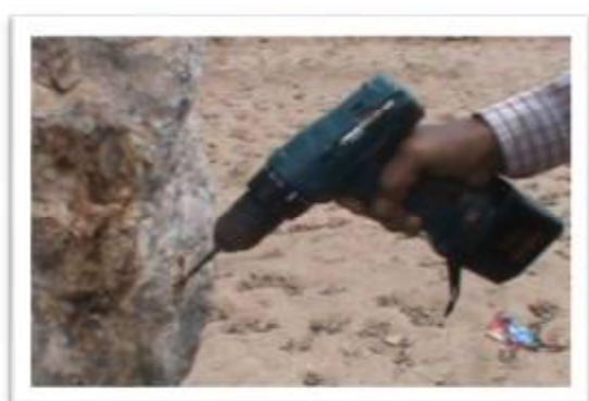
1. Making hole with battery operated drill machine
