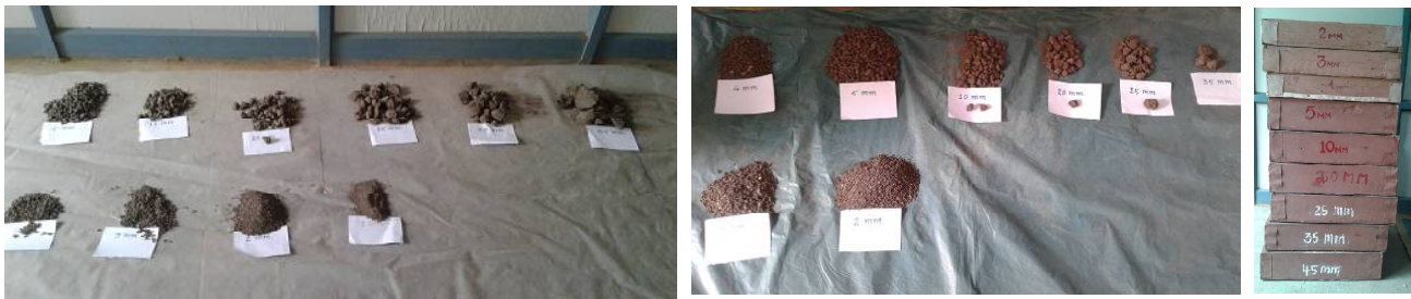
Fig. 5. Soil MWD determination by sieve analysis - horizontal plough (left), vertical plough (center) and sieve.
