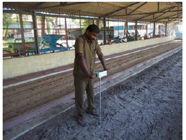
Fig. 4b. Soil cone index measurement
